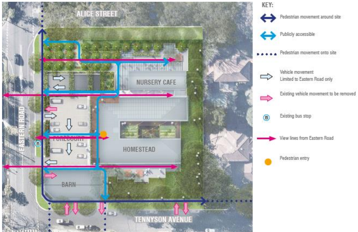
Figure 11: Access and Movement – Circulation Diagram (Source: Urban Design Statement by Oculus, August 2018)
