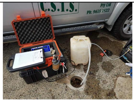
I: Groundwater Sampling Equipment in MW3
